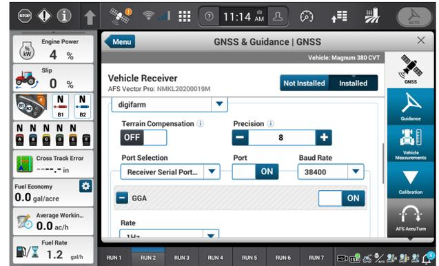
9 Select the satellite icon from the top bar and confirm RTK fix.
