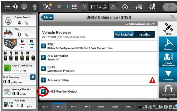
8 Create a new output configuration. Turn Terrain compensation off (this is only for the output, this does not impact the terrain compensation for the steering system). Set your port selection to Receiver Serial Port #1. Turn Port on. Set Baud rate to 38400. Select GGA, Turn it on, set the rate to 1
