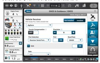
7 Select the satellite icon from the top bar and confirm RTK fix.
