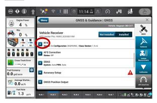
Turn RTK on, Set a new configuration and name. Set the Correction source to RTK External Device. Port setting: Receiver serial port #2. Data parity: None. Baud rate:38400. Stop bits 1. Protocol RTCM 3.
