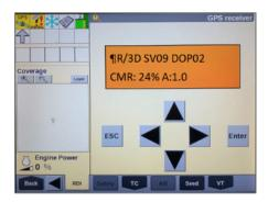
4 On the GPS setup screen, Set the correction type to RTK, Corrections level to AGGPS Radio. Enable the the backup source to xFill, set xFill options to custom>select xFill Setup Edit.
