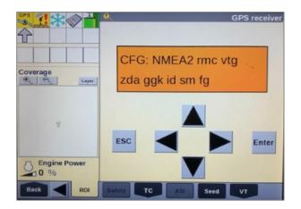
10 Confirm RTK (with a capital R) in the top left hand corner as well as an A:#### in the bottom right. (This can also be confirmed by noticing DGPS in the upper left hand of the full screen)
